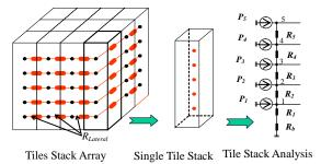
Figure 2. 3-D Compact Resistive Network Thermal Model
