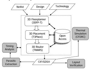
Figure 1. The Proposed 3-D IC Physical Design Flow
