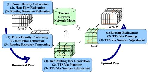
Figure 6. Thermal-Driven 3-D Multilevel Routing System Framework
