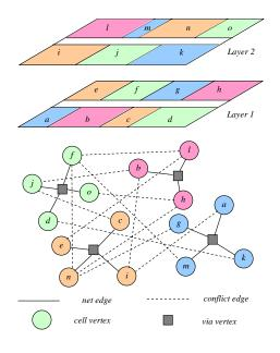
**Figure 5. Relaxed Conflict-Net Graph** We also compared the two transformation methods: LST and folding. Folding can achieve very few TS via numbers — over 90% fewer than those of LST with a cost of 81% longer wirelength.
