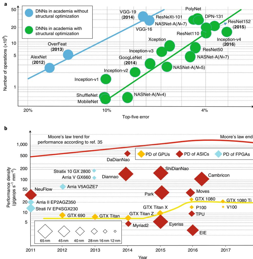
**Fig. 3 | Gap between required number of operations and performance density. a**, Number of operations versus top-five error rate for leading DNN designs from ImageNet classification competition. **b**, Performance density (PD) of leading GPU, ASIC and FPGA platforms. To catch up with the required number of operations, simply increasing the chip area is not feasible. Only the leading DNNs are labelled with a year. The y axis is in log scale. Data taken from refs <sup>1-31,19,20</sup>.
