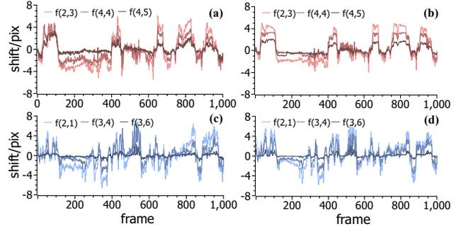
**Figure 4: Extracted motion vectors in horizontal/vertical direction from three different image patches by using the NoRMCorre method (a)/(c) and the LSTM inference (b)/(d).**
