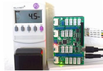
Figure 9: Power measurement of the non-rigid motion correction implementation on the Ultra96 board.
