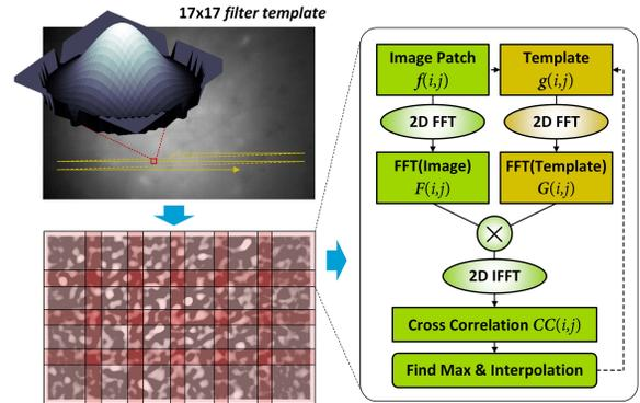
Figure 2: Conventional non-rigid motion detection flow.
