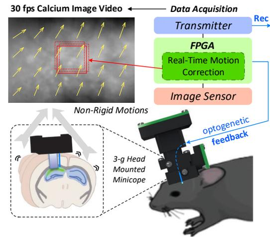
**Figure 1: Real-time non-rigid motion correction for calcium image sensed by head-mounted miniscope [1].**
