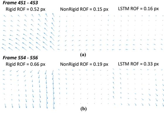
Figure 5: Mean ROF of the motion corrected (a) No.451-453 frames and (b) No.554-556 frames across time by the rigid, non-rigid and LSTM-assisted methods.
