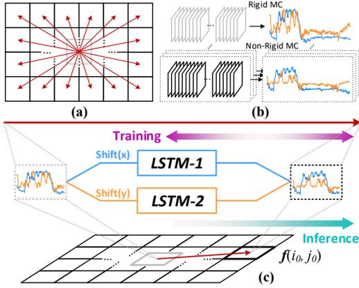
**Figure 3: (a) Proposed LSTM-assisted non-rigid motion correction. (b) Motion vector extraction for the central region and all image patches. (c) LSTM inference on one patch.**
