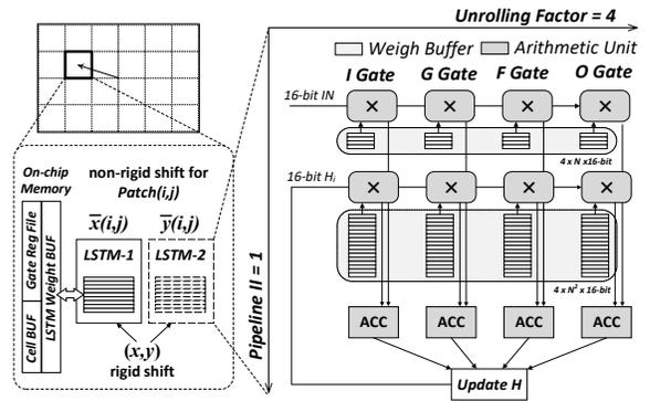
Figure 8: Microarchitecture for the LSTM inference [3].
