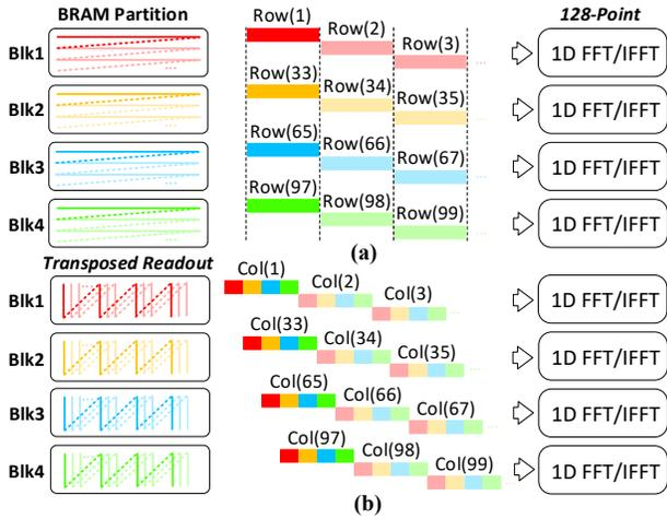
Figure 7: (a) BRAM partition and FFT/IFFT unrolling for row-wise parallel operation, and (b) transposed BRAM readout timing for column-wise parallel FFT/IFFT operations.
