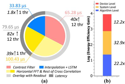
**Figure 10: (a) Breakdown of runtime on FPGA and (b) energy efficiency gain over the CPU implementation.**
