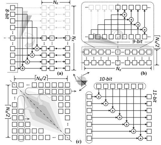
Figure 6: Proposed (a) 1st stage (b) 2nd stage and (c) 3rd stage folding architecture for the contrast filter featuring centrally symmetric coefficients.
