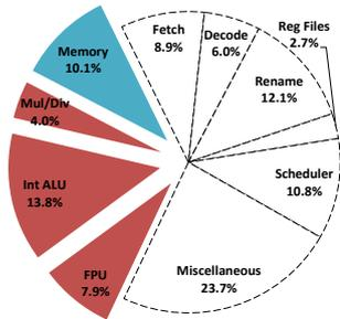
Figure 2: Energy breakdown of original pipeline
