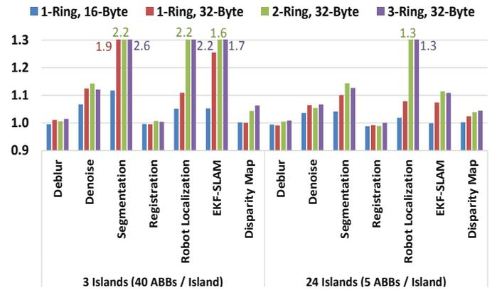
**Figure 7: Performance of various SPM↔DMA ring networks; shown for 3 islands (40 ABBs / island) and 24 islands (5 ABBs / island); normalized to baseline for respective number of islands**
