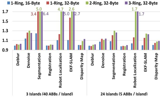
**Figure 8: Performance per unit energy of selected designs; normalized to baseline for respective number of islands**
