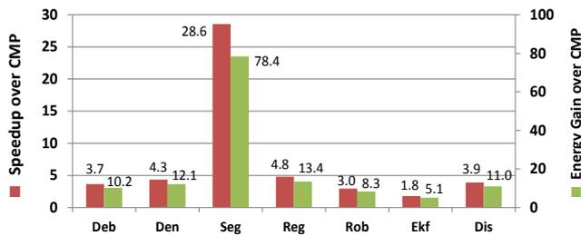
**Figure 10: Performance and energy gains of “best” accelerator-rich design configuration over chip multi-processor (CMP)**
