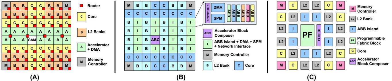
Figure 4: Overview (not to scale) of accelerator-rich architectures: (A) ARC; (B) CHARM; (C) CAMEL
