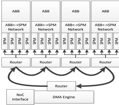
Figure 5: Island design using ring for SPM↔DMA network
