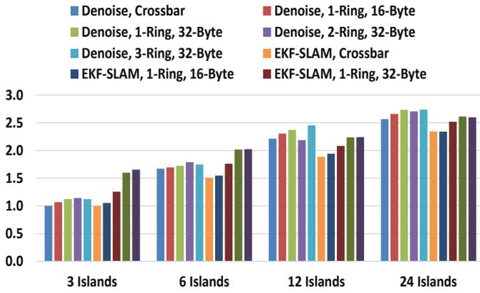
**Figure 6: Performance impact of utilizing different SPM↔DMA networks while adjusting number and size of ABB islands; normalized to baseline for 3 islands**
