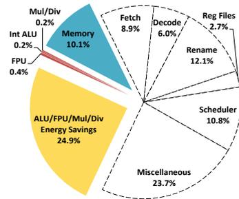
Figure 3: Energy breakdown when custom ASIC is employed
