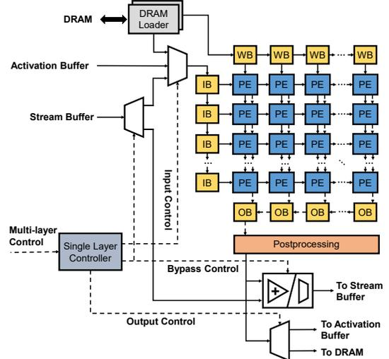
Figure 5: Accelerator design
